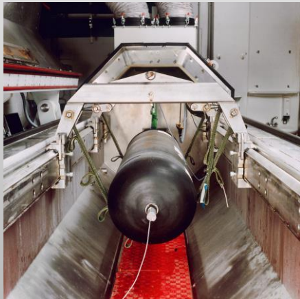
CNG container and respective fatigue test set up (BAM)
