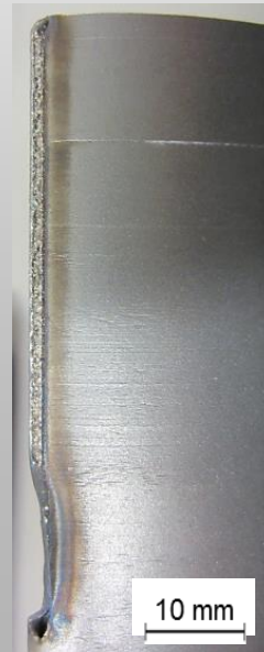
Repair of a turbine blade edge by Laser Powder Welding (LPA)
