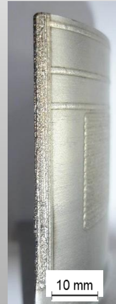
Repair of a turbine blade edge by Laser Powder Welding (LPA)
