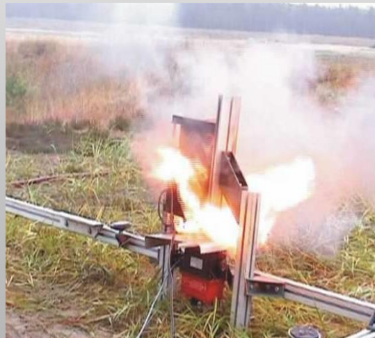
Test set-up to investigate the fire resistance of batteries at accidental penetration (BAM)
