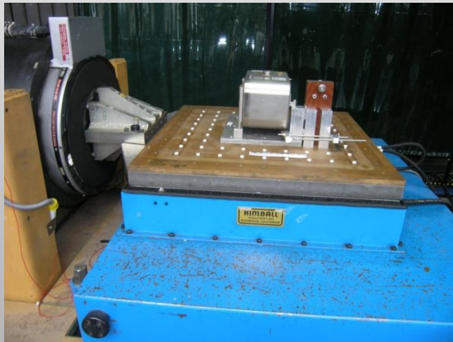
Test set-up to investigate the fatigue resistance of batteries (BAM)
