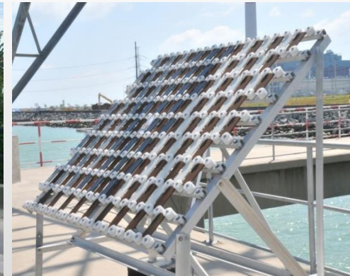
Exposure test of steel specimens in tropical climate (MTec)
