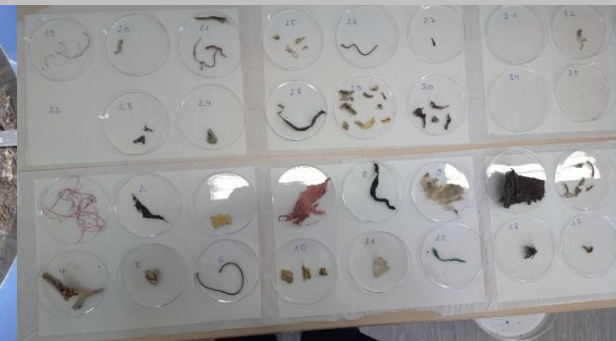
Samples of polymer materials taken from organic waste / compost and prepared for lab investigations (BAM)
