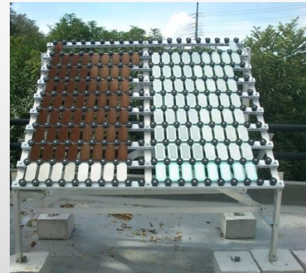
Exposure test of steel specimens in tropical climate (MTec)
