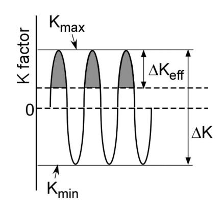
Crack closure factor  $U = \Delta K_{eff} / \Delta K$
