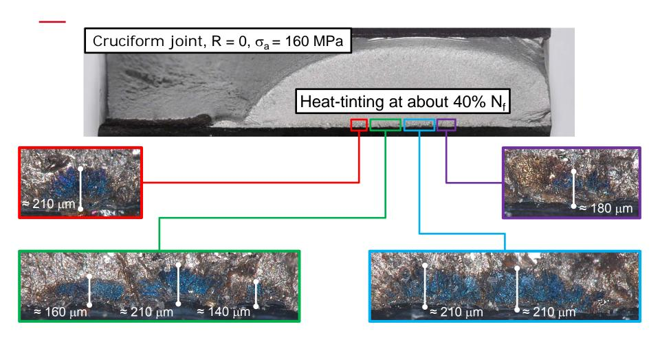
The fatigue life is controlled by the initiation and propagation of short cracks
