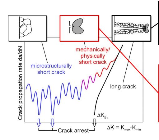
Long crack: small scale yielding holds!  $\Delta K$  can be used to calculate the crack driving force
